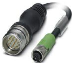
Sensor/actuator cable, 12-position, PUR/PVC, black RAL 9005, shielded, Plug straight M23, coding: A, on Socket straight M12 SPEEDCON, coding: A, cable length: 0.5 m
