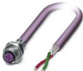
Bus system flush-type socket, PROFIBUS, 2-pos., M12, shielded, B-coded, SPEEDCON, rear/screw mounting with Pg9 thread, with 2.0 m bus cable, 2 x 0.25 mm 2
