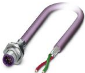
Bus system flush-type plug, PROFIBUS, 2-pos., M12, shielded, B-coded, SPEEDCON, rear/screw mounting with Pg9 thread, with 1.0 m bus cable, 2 x 0.25 mm²
