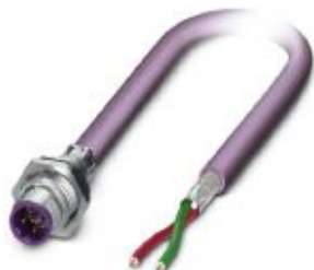
Bus system flush-type plug, PROFIBUS, 2-pos., M12, shielded, B-coded, SPEEDCON, rear/screw mounting with Pg9 thread, with 5.0 m bus cable, 2 x 0.25 mm 2
