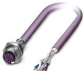
Bus system flush-type socket, DeviceNet/CANopen, 5-pos., M12, shielded, A-coded, Speedcon, rear/screw mounting with Pg9 thread, with 1.0 m bus cable, 2 x 0.2 mm 2 ; 2 x 0.32 mm 2
