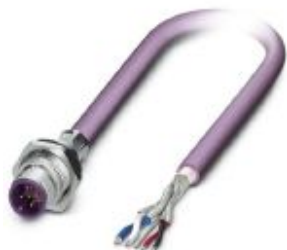
Bus system flush-type plug, DeviceNet/CANopen, 5-pos., M12, shielded, A-coded, SPEEDCON, rear/screw mounting with Pg9 thread, with 5.0 m bus cable, 2 x 0.2 mm 2 , 2 x 0.32 mm 2
