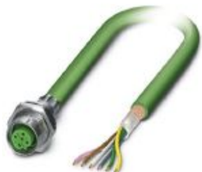
Bus system flush-type female connector, INTERBUS, 5-pos., M12, shielded, B-coded, SPEEDCON, rear/screw mounting with Pg9 thread, with 1.0 m bus line
