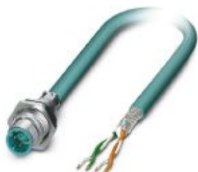
Bus system flush-type plug, Ethernet, 4-pos., M12 SPEEDCON, shielded, D-coded, rear/screw mounting with Pg9 thread, with 1.0 m bus cable, 2 x 2 x 0.2 mm 2
