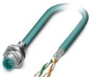
Bus system flush-type plug, Ethernet, 4-pos., M12 SPEEDCON, shielded, D-coded, rear/screw mounting with Pg9 thread, with 2.0 m bus cable, 2 x 2 x 0.2 mm 2
