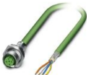
Bus system flush-type socket, PROFINET, 4-pos., M12, shielded, D-coded, SPEEDCON, rear/screw mounting with Pg9 thread, with 0.5 m bus cable, 2 x 2 x 0.34 mm 2
