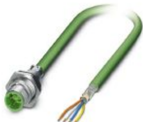
Bus system flush-type plug, PROFINET, 4-pos., M12, shielded, D-coded, SPEEDCON, rear/screw mounting with Pg9 thread, with 1.0 m bus cable, 2 x 2 x 0.34 mm 2
