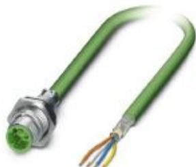
Bus system flush-type plug, PROFINET, 4-pos., M12, shielded, D-coded, SPEEDCON, rear/screw mounting with Pg9 thread, with 5.0 m bus cable, 2 x 2 x 0.34 mm<sup>2</sup>
