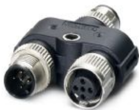
Y distributor, 5-position, shielded, Plug straight M12 SPEEDCON, coding: A, on Socket straight M12 SPEEDCON, coding: A and Plug straight M12 SPEEDCON, coding: A, Parallel distributor
