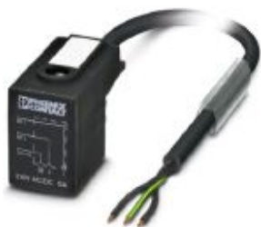
Sensor/actuator cable, 3-position, PUR halogen-free, black-gray RAL 7021, free cable end, on Valve connector BI (11 mm), cable length: 10 m
