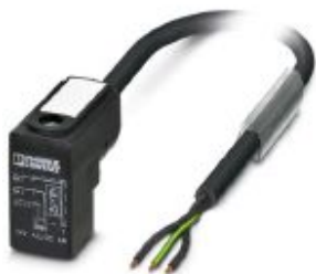
Sensor/actuator cable, 3-position, PVC, black RAL 9005, free cable end, on Valve connector C (8 mm), with 1 LED, connected with Z diode, cable length: 1.5 m
