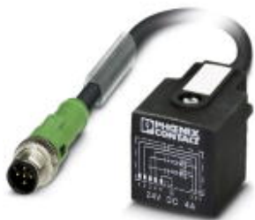
Sensor/actuator cable, 5-position, PUR halogen-free, black-gray RAL 7021, Plug straight M12, A-coded, on Valve connector AD (pressure switch), with 2 LEDs, cable length: 0.6 m
