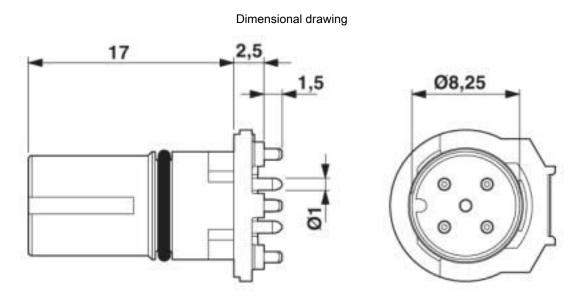
M12 female connector contact carrier
