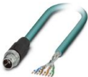
Assembled Ethernet cable, CAT6 A , shielded, 4-pair, AWG 26 stranded (7-wire), RAL 5021 (water blue), M12 plug on free conductor end, length 5 m
