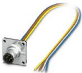
Sensor/actuator flush-type plug, 4-pos., M12, D-coded, front/square flange mounting, with 0.5 m TPE litz wire, 4 x 0.34 mm 2
