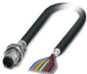
Flush-type plug, shielded, 12-pos., M12, A-coded, rear/screw mounting with M16 thread, with 2 m cable, 12 x 0.14 mm 2
