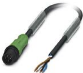
Sensor/actuator cable, 4-position, PUR halogen-free, black-gray RAL 7021, Plug straight M12, coding: A, on free cable end, cable length: 1.5 m, with plastic knurl
