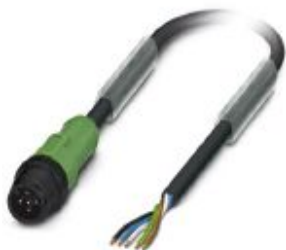
Sensor/actuator cable, 5-position, PUR halogen-free, black-gray RAL 7021, Plug straight M12, coding: A, on free cable end, cable length: 1.5 m, with plastic knurl
