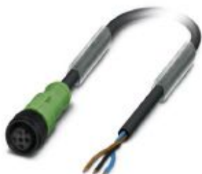
Sensor/actuator cable, 3-position, PUR halogen-free, black-gray RAL 7021, free cable end, on Socket straight M12, coding: A, cable length: 1.5 m, with plastic knurl
