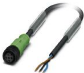
Sensor/actuator cable, 3-position, PUR halogen-free, black-gray RAL 7021, free cable end, on Socket straight M12, coding: A, cable length: 10 m, with plastic knurl
