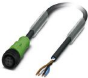
Sensor/actuator cable, 4-position, PUR halogen-free, black-gray RAL 7021, free cable end, on Socket straight M12, coding: A, cable length: 5 m, with plastic knurl
