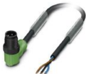
Sensor/actuator cable, 3-position, PUR halogen-free, black-gray RAL 7021, Plug angled M12, coding: A, on free cable end, cable length: 1.5 m, with plastic knurl
