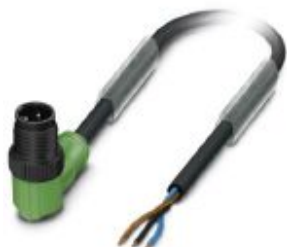
Sensor/actuator cable, 3-position, PUR halogen-free, black-gray RAL 7021, Plug angled M12, coding: A, on free cable end, cable length: 10 m, with plastic knurl
