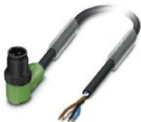
Sensor/actuator cable, 4-position, PUR halogen-free, black-gray RAL 7021, Plug angled M12, coding: A, on free cable end, cable length: 1.5 m, with plastic knurl
