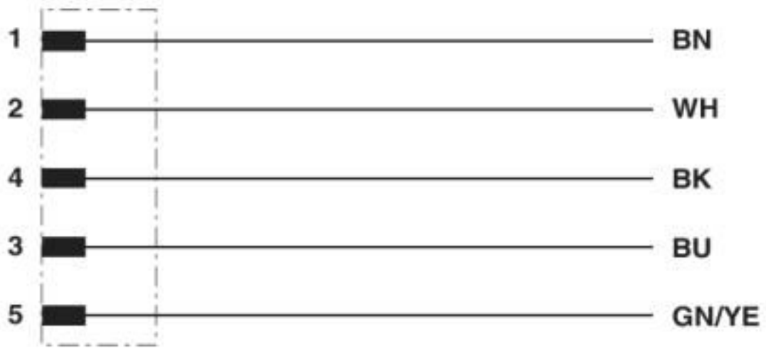
Contact assignment of the M12 plug
