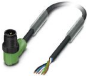
Sensor/actuator cable, 5-position, PUR halogen-free, black-gray RAL 7021, Plug angled M12, coding: A, on free cable end, cable length: 10 m, with plastic knurl
