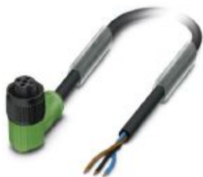
Sensor/actuator cable, 3-position, PUR halogen-free, black-gray RAL 7021, free cable end, on Socket angled M12, coding: A, cable length: 3 m, with plastic knurl
