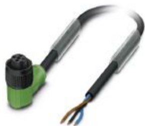
Sensor/actuator cable, 3-position, PUR halogen-free, black-gray RAL 7021, free cable end, on Socket angled M12, coding: A, cable length: 5 m, with plastic knurl
