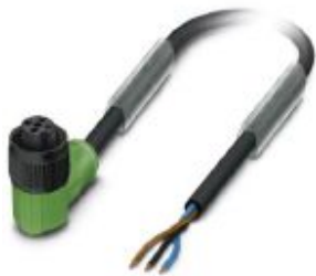
Sensor/actuator cable, 3-position, PUR halogen-free, black-gray RAL 7021, free cable end, on Socket angled M12, coding: A, cable length: 10 m, with plastic knurl
