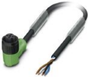
Sensor/actuator cable, 4-position, PUR halogen-free, black-gray RAL 7021, free cable end, on Socket angled M12, coding: A, cable length: 10 m, with plastic knurl
