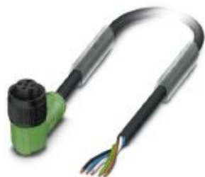
Sensor/actuator cable, 5-position, PUR halogen-free, black-gray RAL 7021, free cable end, on Socket angled M12, coding: A, cable length: 1.5 m, with plastic knurl
