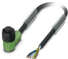
Sensor/actuator cable, 5-position, PUR halogen-free, black-gray RAL 7021, free cable end, on Socket angled M12, coding: A, cable length: 10 m, with plastic knurl
