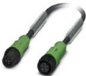
Sensor/actuator cable, 5-position, PUR halogen-free, black-gray RAL 7021, Plug straight M12, coding: A, on Socket straight M12, coding: A, cable length: 3 m, with plastic knurl
