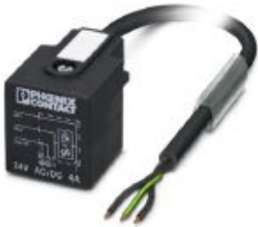
Sensor/actuator cable, 3-position, PUR halogen-free, black-gray RAL 7021, free cable end, on Valve connector A, with 1 LED, connected with Varistor, cable length: 10 m
