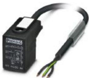
Sensor/actuator cable, 3-position, PUR halogen-free, black-gray RAL 7021, free cable end, on Valve connector B (10 mm), with 1 LED, connected with Varistor, cable length: 3 m
