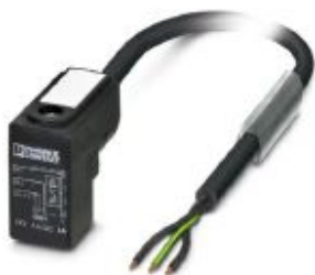
Sensor/actuator cable, 3-position, PUR halogen-free, black-gray RAL 7021, free cable end, on Valve connector C (8 mm), with 1 LED, connected with Varistor, cable length: 1.5 m
