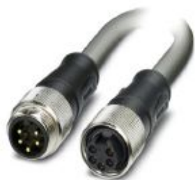
Power cable, 5-position, PVC, gray RAL 7001, Plug straight 7/8"-16UNF, coding: A, on Socket straight 7/8"-16UNF, coding: A, cable length: 2 m, 1.5 mm 2 conductor cross section, For power supply
