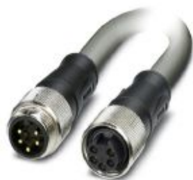
Power cable, 5-position, PVC, gray RAL 7001, Plug straight 7/8"-16UNF, coding: A, on Socket straight 7/8"-16UNF, coding: A, cable length: 0.3 m, 2.5 mm 2 conductor cross section, For power supply
