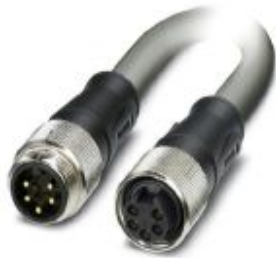
Power cable, 5-position, PVC, gray RAL 7001, Plug straight 7/8"-16UNF, coding: A, on Socket straight 7/8"-16UNF, coding: A, cable length: 2 m, 2.5 mm 2 conductor cross section, For power supply
