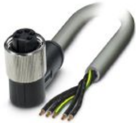
Power cable, 5-position, PUR, gray RAL 7001, free cable end, on Socket angled 7/8"-16UNF, cable length: 3 m, 1.5 mm 2 conductor cross section, For power supply
