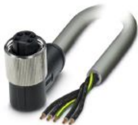
Power cable, 5-position, PUR, gray RAL 7001, free cable end, on Socket angled 7/8"-16UNF, cable length: 10 m, 1.5 mm 2 conductor cross section, For power supply
