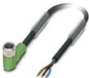
Sensor/actuator cable, 3-position, PVC, black RAL 9005, free cable end, on Socket angled M8, cable length: 3 m
