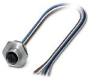
Sensor/actuator flush-type socket, 5-pos., M12, A-coded, front/screw mounting with M20 x 1.5 thread, with 0.5 m TPE litz wire, 5 x 0.34 mm 2 , high-grade steel version
