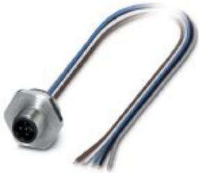
Sensor/actuator panel-mount connector, 5-pos., M12, B-coded, front/screw mounting with M20 x 1.5 thread, with 0.5 m TPE litz wire, 5 x 0.34 mm 2 , stainless steel version
