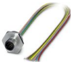
Sensor/actuator flush-type plug, 8-pos., M12, A-coded, front/screw mounting with M20 x 1.5 thread, with 0.5 m TPE litz wire, 8 x 0.25 mm 2 , high-grade steel version
