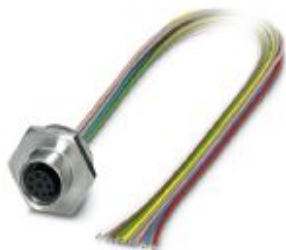
Sensor/actuator flush-type socket, 8-pos., M12, A-coded, front/screw mounting with M20 x 1.5 thread, with 0.5 m TPE litz wire, 8x 0.25 mm 2 , high-grade steel version
